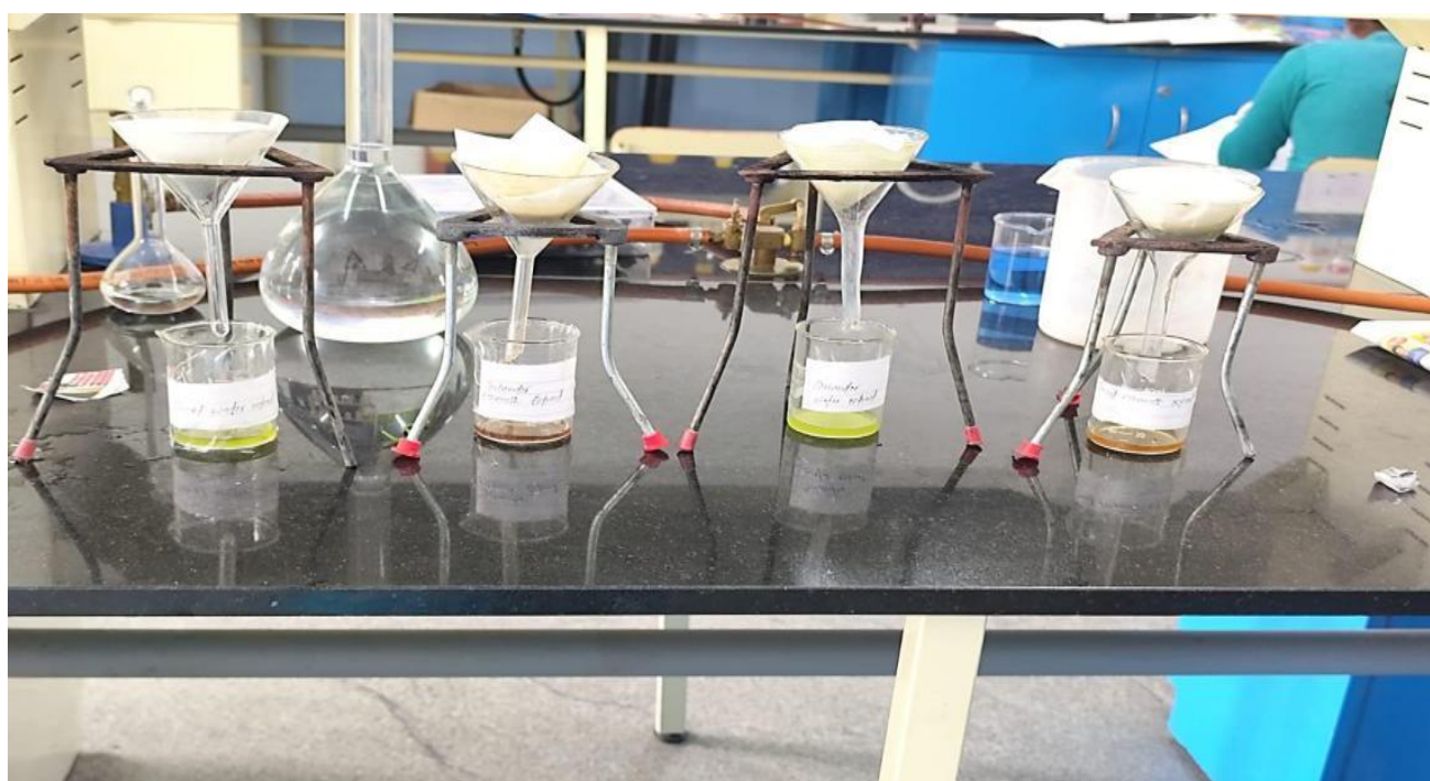
Figure 2: Preparation of herbal extracts of fennel and coriander for qualitative phytochemical screening. Determination of Volatile Oil Content
