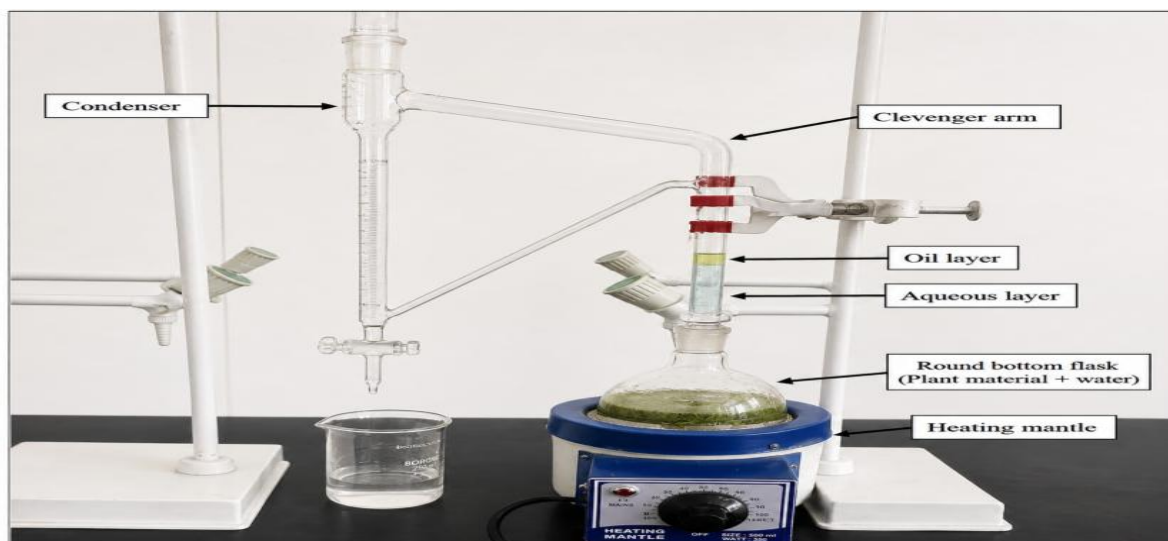
Figure 3: Determination of volatile oil content of herbal materials using Clevenger apparatus by steam distillation.
