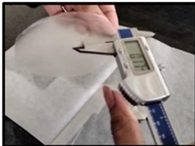
Figure 5: Measurement of thickness of the buccal film
