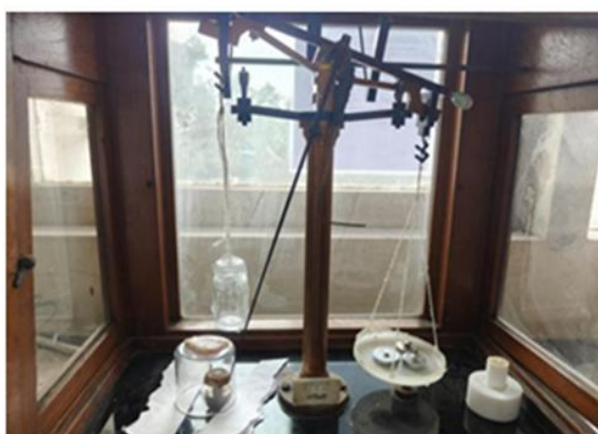
Figure 6: Mucoadhesion Testing using a Modified Physical Balance
