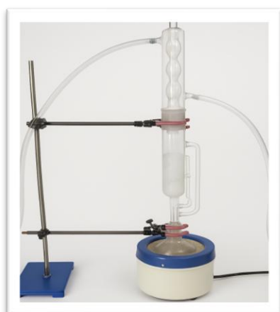
Figure 2.2.1 Construction of Soxhlet apparatus
