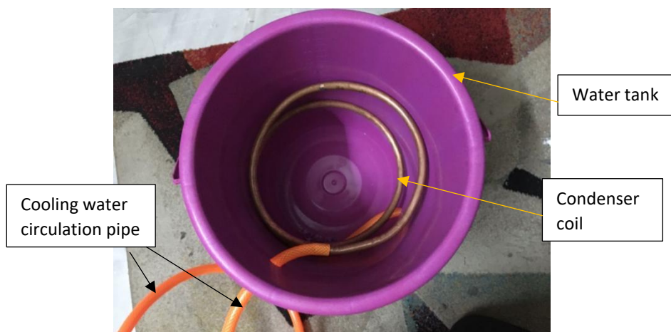
Figure 23: Water-cooled condenser used to condense cow urine vapour generated by a pressure cooker (Top view)
