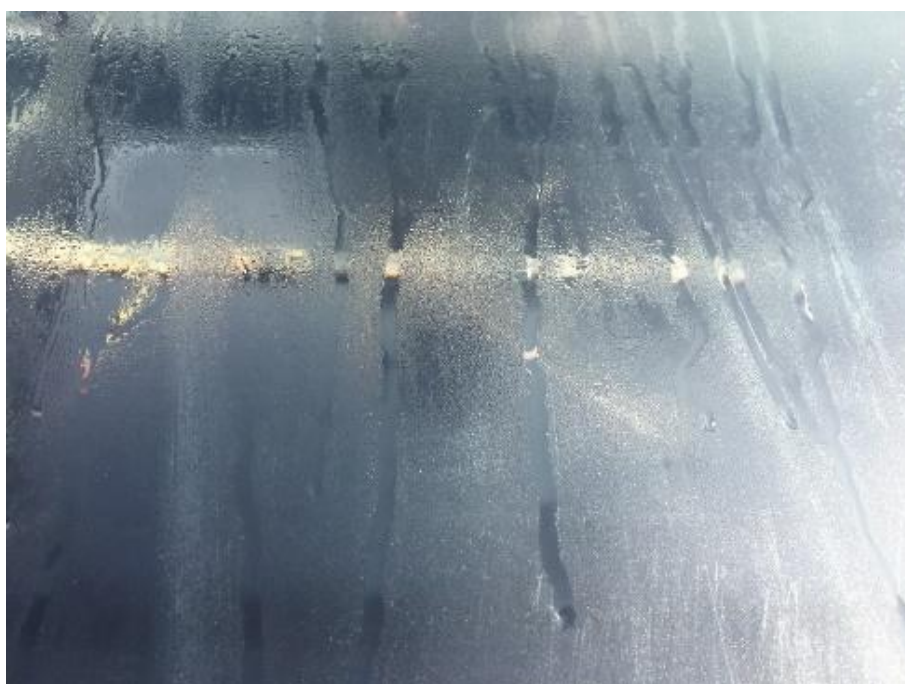
Figure 13: Condensation of cow urine vapour, underside of the glass cover, which is called cow urine distillate
