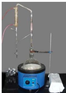
Figure 4: Production of cow urine distillate using a glass apparatus
