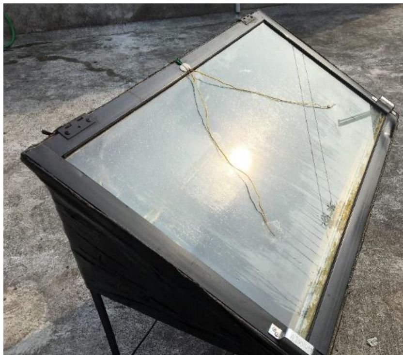
Figure 12: Photograph of a fabricated solar thermal hydrodistiller for cow urine distillation (Glassdoor closed)
