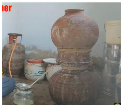
Figure 5: Production of cow urine distillate using the spherical clay pot apparatus
