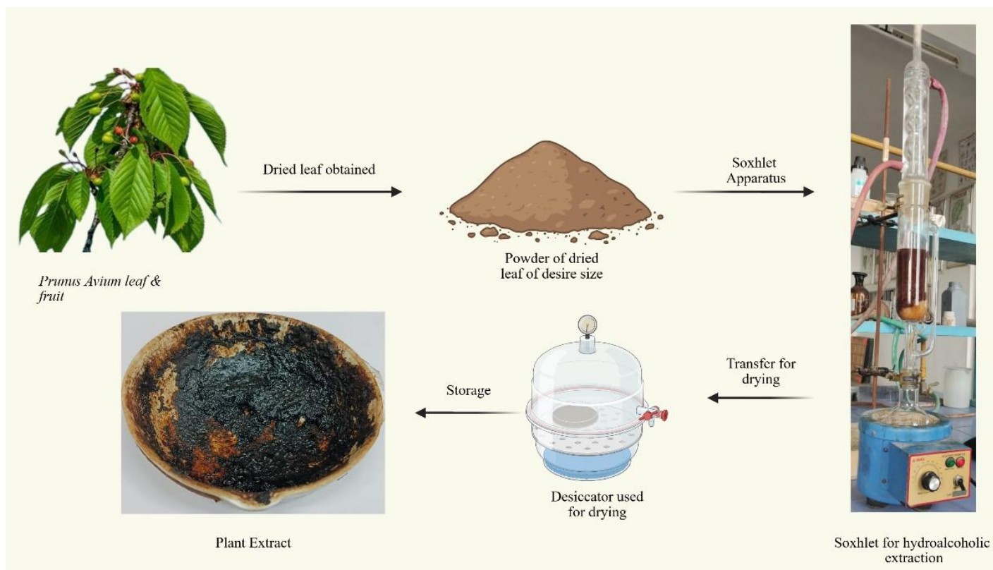
Figure 1: Extraction process of Prunus avium leaves extract. https://BioRender.com
