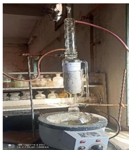
Figure 2: Extraction of Lantana camara Leaves powder by Soxhlet Apparatus
