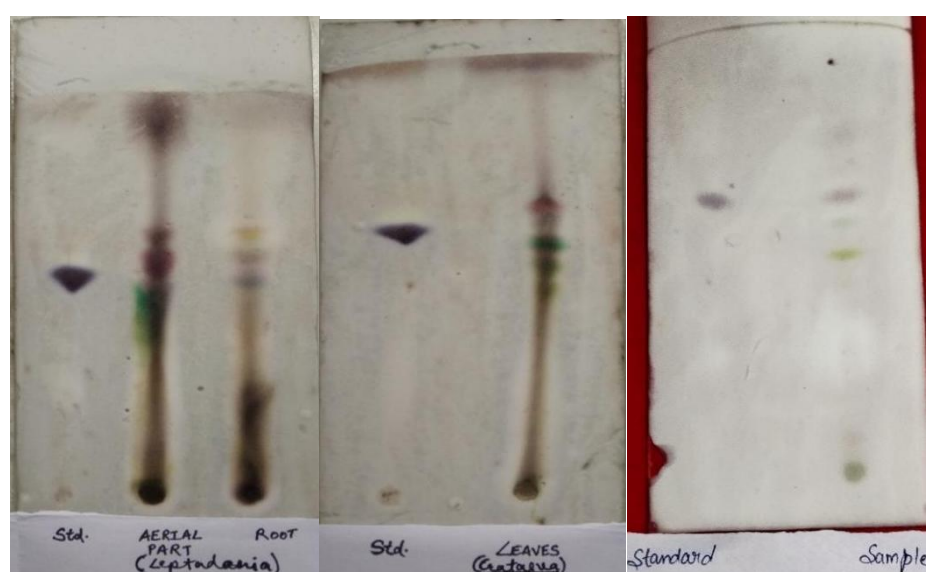
Figure 1: Chromatographic characteristics of Phytosterol compounds isolated from (A) L. pyrotechnica aerial and root part (B) C. nurvala leaf and (C) C. nurvala fruit
