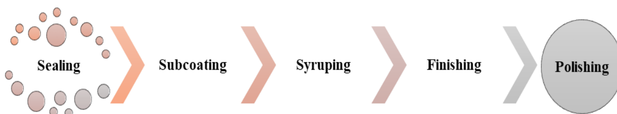
Figure 2: Representation of steps of tablet coating and tablet finished products
