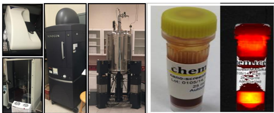
Figure 1: A Zetasizer; B: Sonicator; C: PerkinElmer IVIS Spectrum imaging system; D: Bruker MRI; E: vial of nanoparticles; F: vial of the nanoparticle as imaged under PerkinElmer IVIS system
