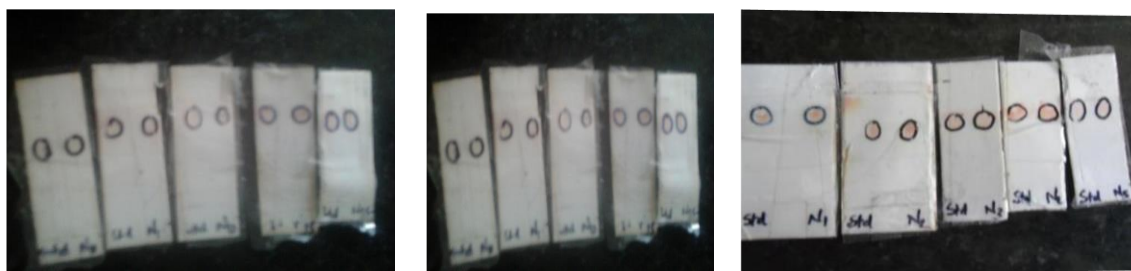
Figure 6: Chemical characterization of Clindamycin hydrochloride - excipients mixture at different storage conditions (a) 5 ° ±3 °C (b) 25 ° ±2 °C (c) 40 ° ±2 °C
