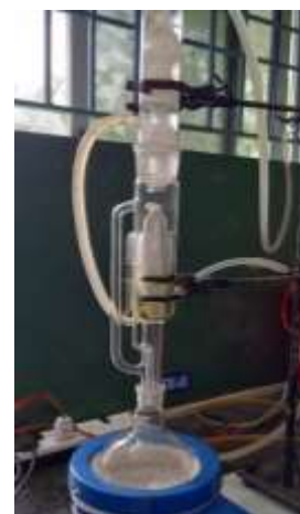
Figure (1b): Solvent extraction by Soxhlet
