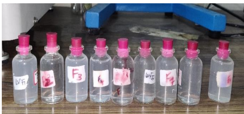
Figure 7 PCP nanosuspension obtained by high energy microfluidization
