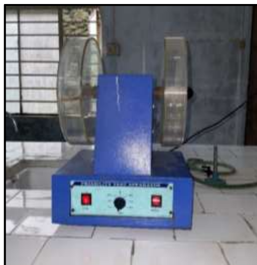
Figure 12: Roche Friabilator for friability check
