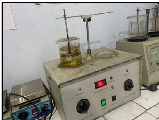
Figure 11: Disintegration time checking by disintegration apparatus
