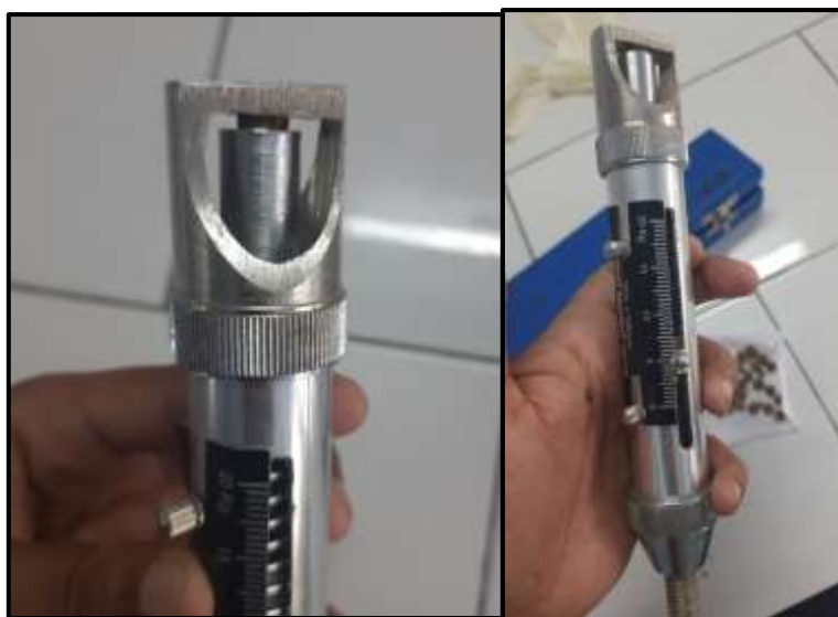
Figure 10: Hardness checking by Monsanto hardness tester
