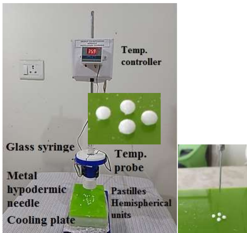
Figure 4: In house Labscale Melt solidification apparatus
