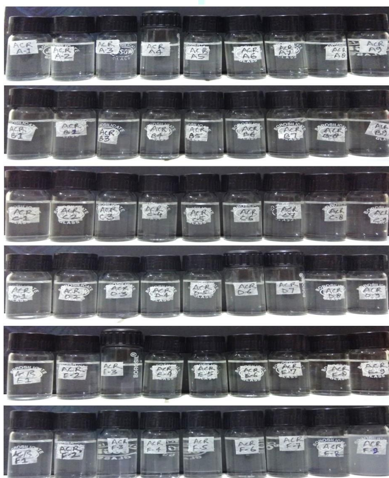
Figure 3: Visual assessment ACR based formulation after assessment of self-emulsification grading
