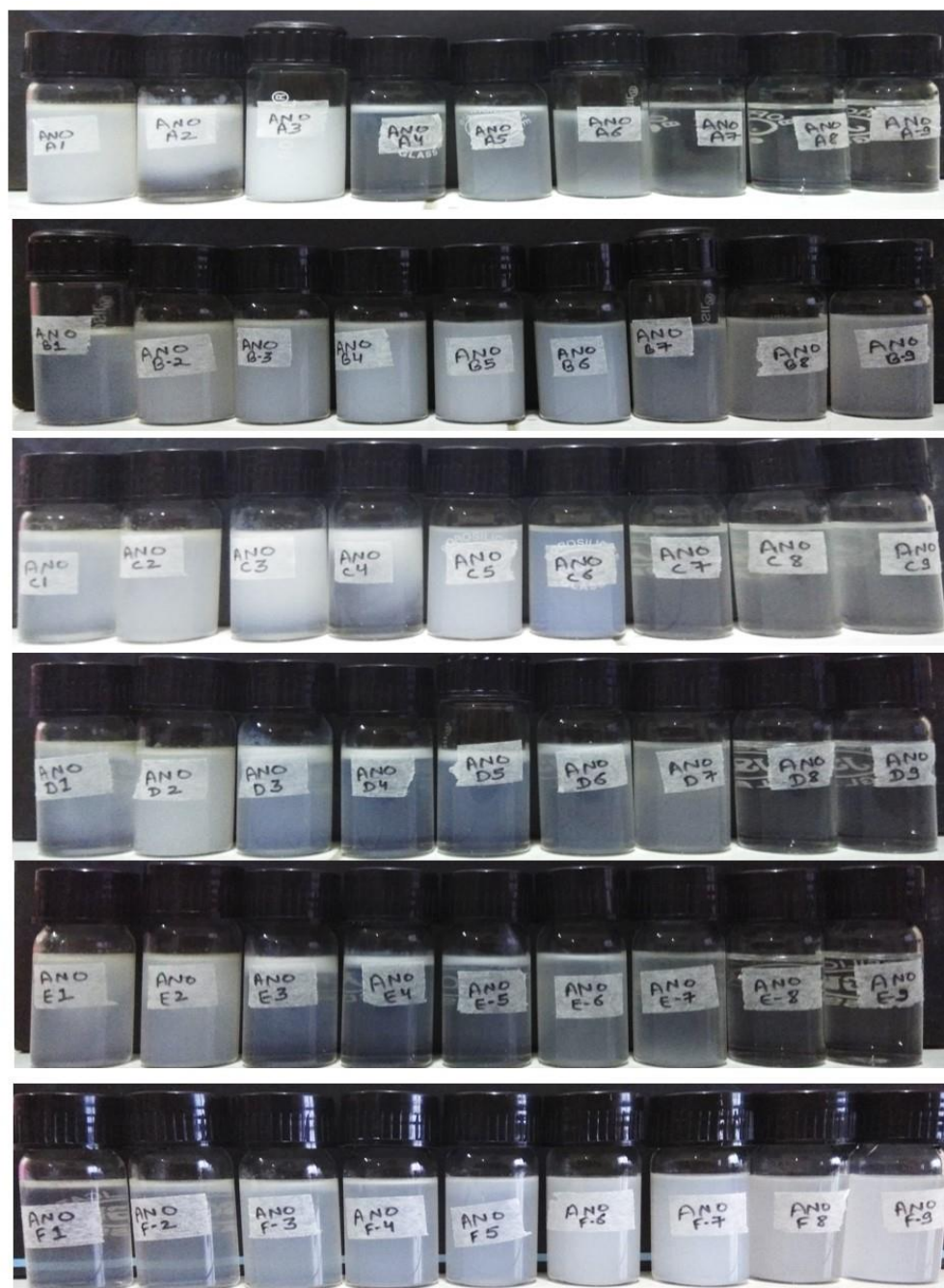
Figure 4: Visual assessment ANO based formulation after assessment of self-emulsification grading
