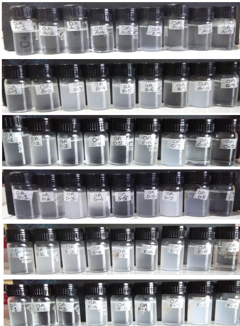
Figure 5: Visual assessment OA based formulation after assessment of self-emulsification grading
