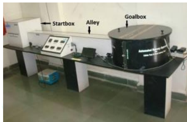
Figure 1: Automated runway apparatus to assess sexual motivation in rats.
