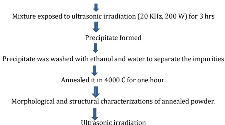
NiO nanoparticles suspended in ethylene glycol (uniform suspension obtained)
