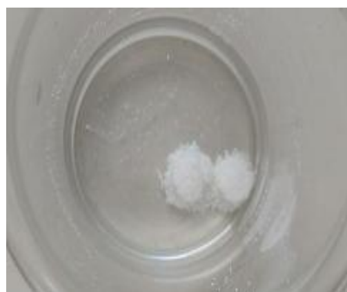
Figure 3: Dispersion test for Methylprednisolone dispersible tablets
