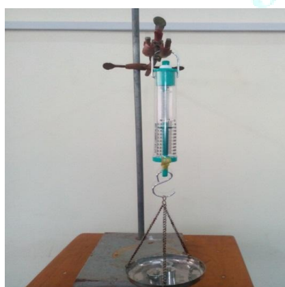
Figure 1: Locally designed Tensile strength and Percent elongation tester
