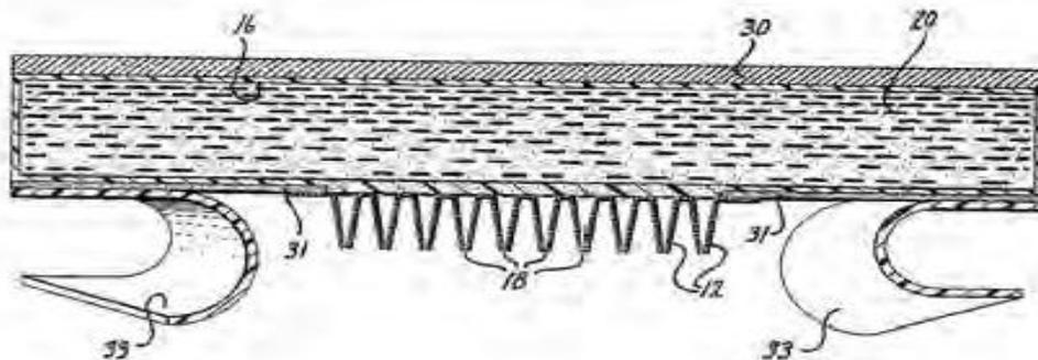
Figure 2: The original concept of a microneedle-based transdermal patch from the patent of Gerstel and Place 1976<sup>22</sup>. The device contains microneedles<sup>12</sup>, a drug reservoir<sup>16</sup>, adhesives<sup>31</sup> and optionally a rate-controlling membrane.
