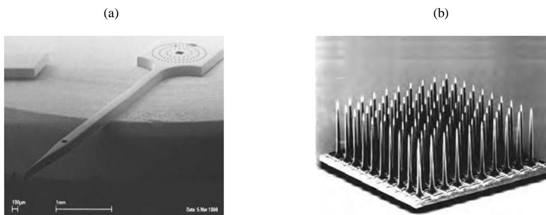
Figure 3: (a) 6 mm long, hollow, in-plane microneedle. From Talbot and Pisano<sup>23</sup>. (b) Individually addressable, 1.5 mm long, solid, out-of-plane microneedles used as electrodes. From Campbell et al.<sup>24</sup>
