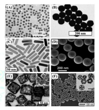
Figure1: SEM images of different AuNP sizes and shapes used in biomedical. (A) 15 nm nanospheres using (B) 150 nm spheres (C) nanorods, (D) nanoshells, (E) cubic nanocages (F) nanocages.
