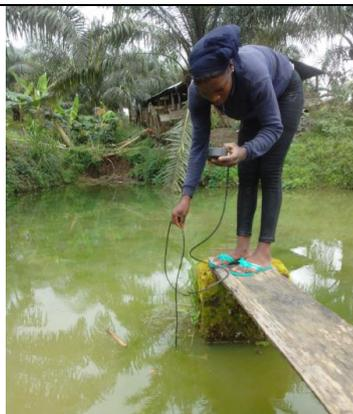
**Figure 1** : Temperature and oxygen measurement in pond E1
