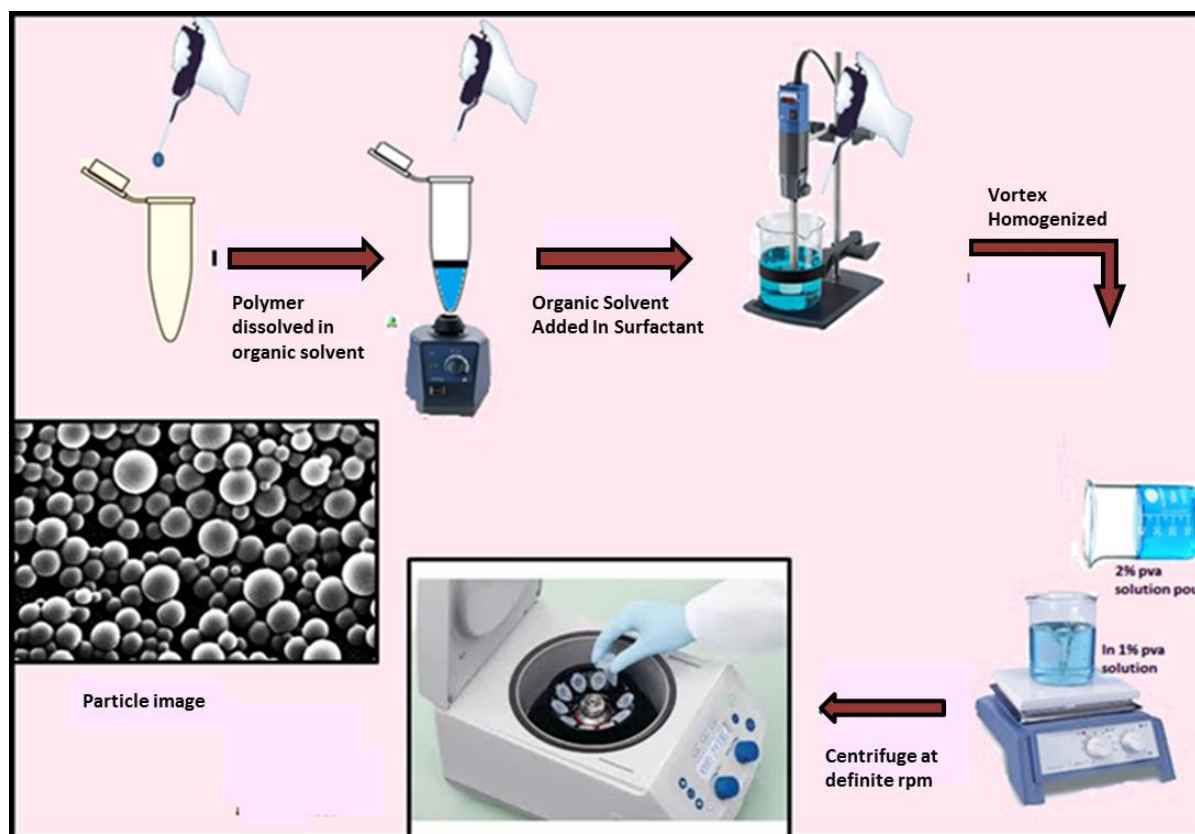
Fig: 4 Representation of double emulsion solvent evaporation method
