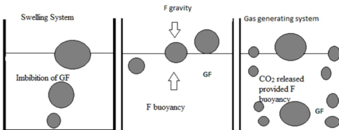
Mechanism of floating system, GF = Gastric fluid
