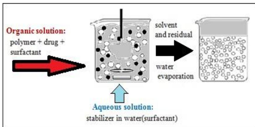
Figure 1: Schematic representation of the solvent displacement technique
