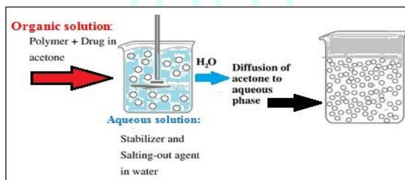
Figure 2: Schematic representation of the salting out technique
