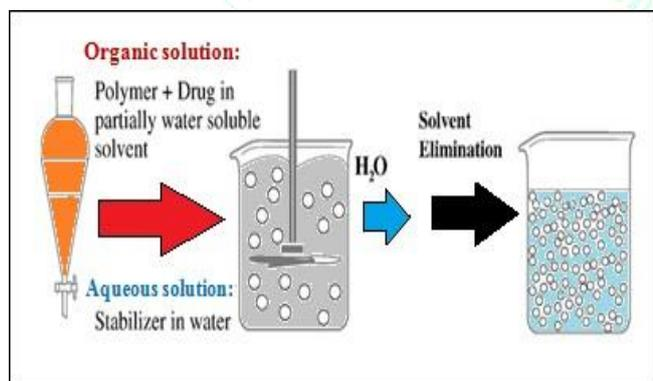
Figure 4: Schematic representation of the emulsification/solvent diffusion technique
