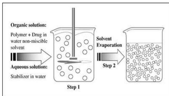
Figure 3: Schematic representation of the solvent-evaporation technique.
