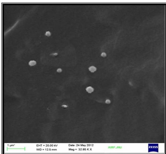
**Figure 2: SEM analysis of SLNs of aceclofenac at magnification 32.85 KX**
