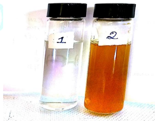
Figure 1: 0.01 M Silver Nitrate is added to 100mL Distilled Water, Vigorously Stirred under 80° C, and 2). Guava leaf Extract being Added Drop Wise
