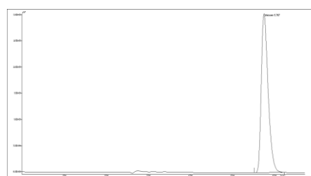
Figure 3: Typical RP- HPLC Chromatogram Brimonidine Tartrate (40 µg/ml) with corresponding retention time.
