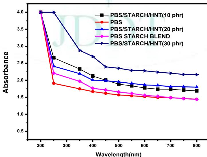
Figure 3: UV study of the PBS, PBS/Starch blend and PBS/Starch/HNT filled composites.
