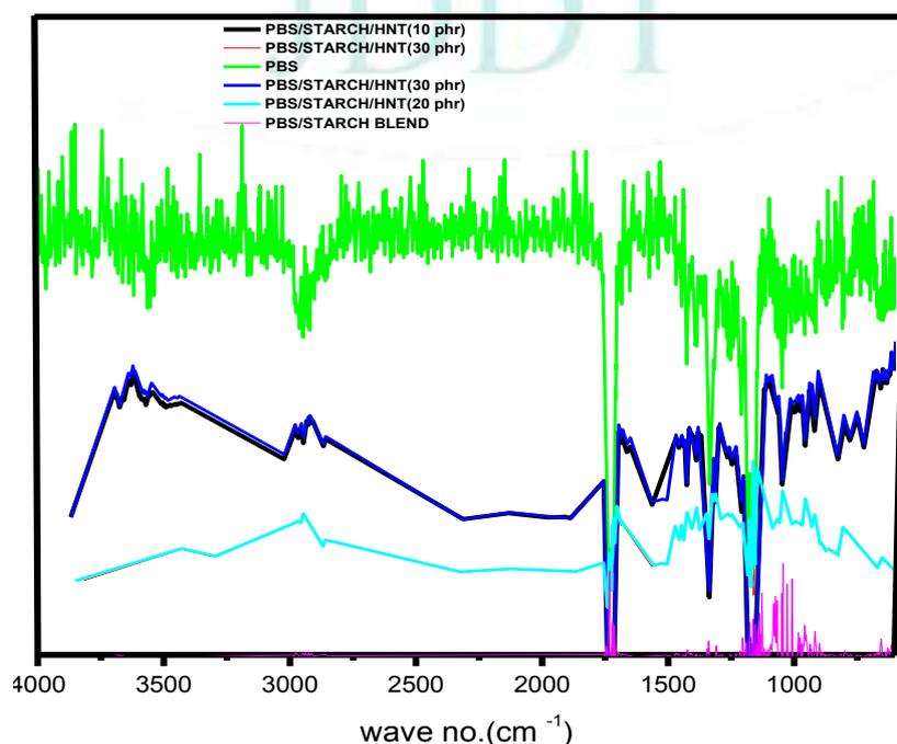
Figure 1: FTIR Analysis of PBS/Starch/Halloysite composites
