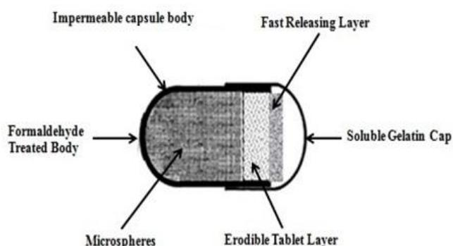
**Figure 1: Overview of designed pulsatile device**
