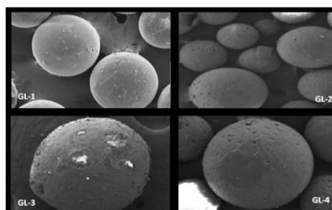
Figure 2: Scanning Electron Micrographs of glipizide microspheres
